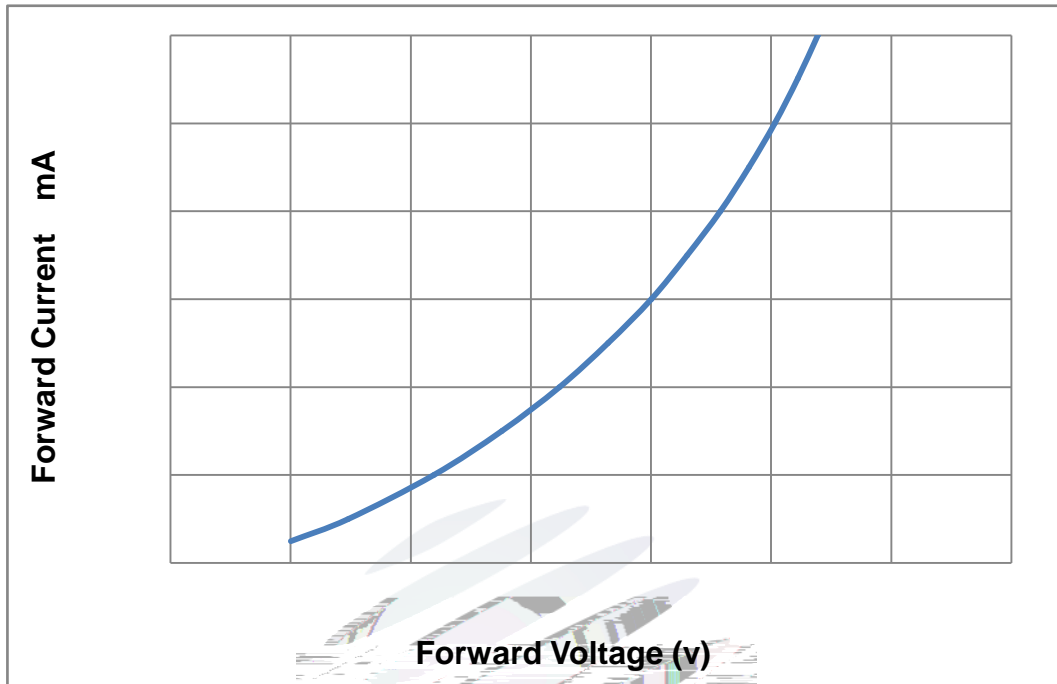
Fig. 1-7 Forward Voltage Vs Forward Current 伏安特性曲线
