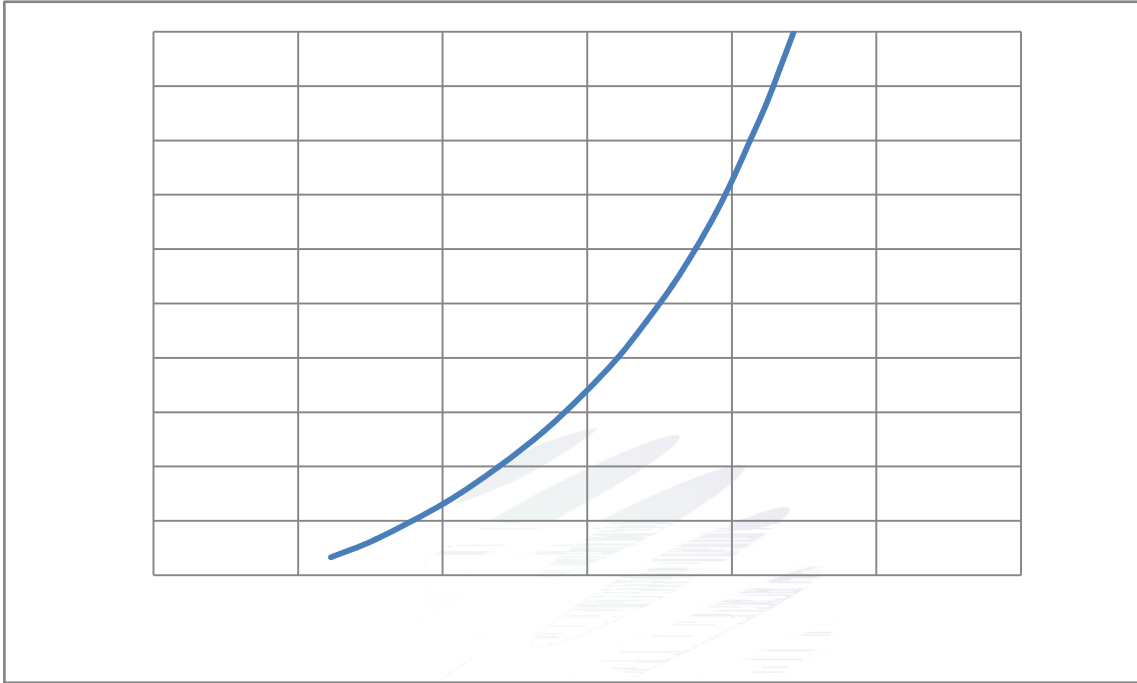
Fig. 1-7 Forward Voltage Vs Forward Current
