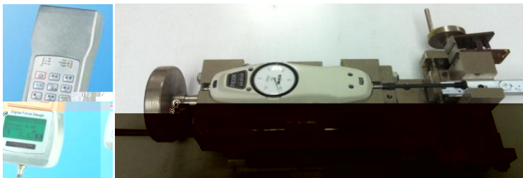
Fig 5-1 Push & Pull Test Equipment
