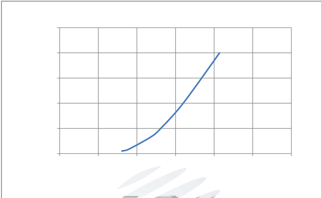
Fig. 1-7 Forward Voltage Vs Forward Current
